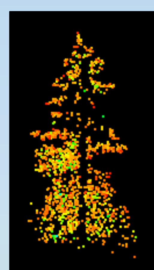
Figure 3a. Georegistered terrestrial laser scanner (TLS) point cloud of spruce "seedlings" <2m tall amongst Betula sp. (dwarf birch) and Alnus sp. (alder) shrubs from TLS scans. A Leica C10 instrument was used for all scans, and each plot was scanned from 4-5 scan positions. Figure 3b. Profile of individual spruce "seedling" from TLS scans.
